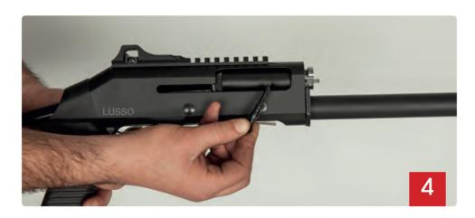
By turning the cocking handle, pull and remove.
