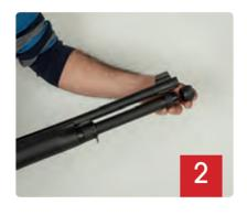
Remove the nut in the magazine tube.
