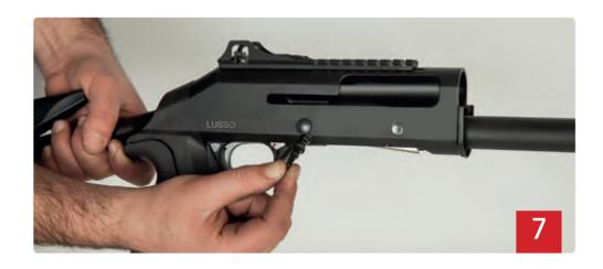
Remove the pin in illustration with the help of the cocking handle(Remove the trigger guard.)
