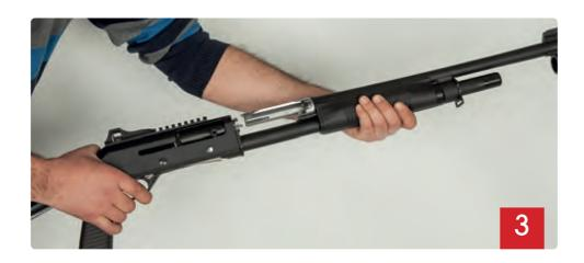
By holding the forend, remove the barrel forward.
